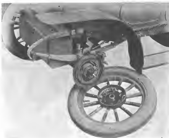
Rear Springs and Brakes, Pierce 4-24 and 6-36 Models.
